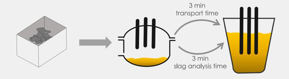
last EAF sample provides precise initial information for desulfurization process in the LF
